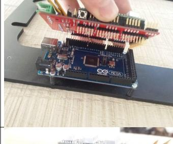
Once you are happy that all of the pins are in place, press down on all edges of the Ramps board to ensure good connections are made.
