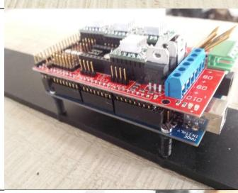
This is what your Ramps and Arduino assembly should look like when pressed together properly. Check all sides are properly connected.
